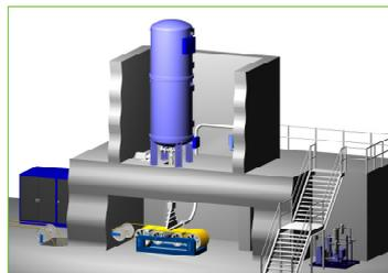
Figure 8. A Dynamitron® 3.0 MeV concrete shielded system for electron beam processing of medium and large size insulated wire, cable and plastic tubing.
