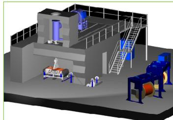
Figure 7. A Dynamitron® 1.5 MeV concrete shielded system for electron beam processing of medium and large size insulated wire, cable and plastic tubing.
