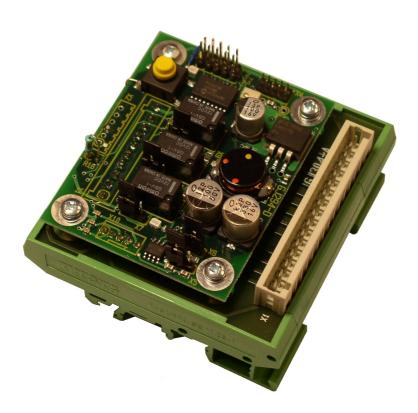
GP-AMP is designed to detect a wide range of gases and vapours. The amplifier has three potential free relay outputs with common arm: relays for Alarm1 (low alarm) and Alarm2 (high alarm) and a fault relay.
