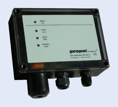
The Geopal GP-SA-2 is a 230VAC version of our well-known GP-SA stand-alone detector. The GP-SA-2 detector uses an integrated microprocessor for continuously monitoring the gas concentration, whether it is in the 0-100% LEL range (lower explosion level) or the 0-40,000 ppm range, in connection with e.g. refrigerants.
