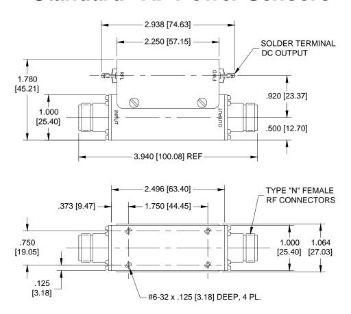
These Directional RF Power Sensors provide DC currents proportional to the Forward and Reflected power flowing through the line. All models are designed to drive a 30 microampere, 1400 ohm meter, or approximately 100 millivolts across a 5K load. Directivity is typically 25 dB minimum. Special calibration is also available.
